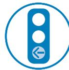
Provides a protected green arrow phase for left turning vehicles while showing a red light for both on-coming traffic and parallel pedestrian crossings. Eliminates conflicts between pedestrians and left-turning vehicles.
