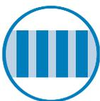
A crosswalk that is designed to be more visible to approaching drivers. Crosswalks should be designed with continental markings and use high-visibility material, such as inlay tape or thermoplastic tape instead of paint.
