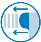
Widens the sidewalk at intersections or midblock crossings to shorten the pedestrian crossing distance, to make pedestrians more visible to vehicles, and to reduce the speed of turning vehicles.
