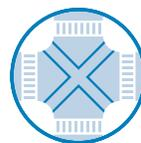
A form of pedestrian “WALK” phase at a signalized intersection in which all vehicular traffic is required to stop, allowing pedestrians to safely cross through the intersection in any direction, including diagonally.
