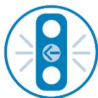
Flashing yellow turn arrow alerts drivers to proceed with caution and decide if there is a sufficient gap in oncoming traffic to safely make a turn. To be used only when a pedestrian walk phase is not called. Protected-only phases should be used when pedestrians are present.
