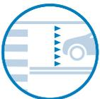
Yield lines are placed 20 to 50 feet in advance of multi-lane pedestrian crossings to increase visibility of pedestrians. Used in conjunction with Yield to Pedestrian signage. Can reduce the likelihood of a multiple-threat crash.
