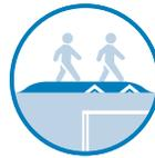
The crosswalk is elevated to match the sidewalk to make pedestrians more visible to approaching vehicles. Typically located at midblock crossings or across free right turns, they encourage motorists to yield to pedestrians and reduce vehicle speed. An entire intersection may be raised similarly.
