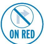
Prohibiting right-run-on-red movements should be considered at skewed intersections, or where exclusive pedestrian "WALK" phases, Leading Pedestrian Intervals (LPIs), sight distance issues, or high bike/ped volumes are present. Can help prevent crashes between vehicles turning right on red from one street and through vehicles on the cross street, and crashes involving bicyclists and pedestrians.
