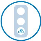
A traffic signal directing bicycle traffic across an intersection. Separates bicycle movements from conflicting motor vehicle, streetcar, light rail, or pedestrian movements. May be applicable for Class IV facilities when the bikeway is brought up to the intersection.
