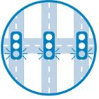
Interconnected signal systems provide coordination between adjacent signals to better facilitate travel through a corridor. When implemented, the number of stops is reduced, and therefore the opportunity to run red lights is also reduced.
