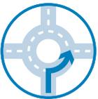
Roundabouts are circular intersections designed to eliminate left turns by requiring traffic to travel in a counter-clockwise direction and exit to the right. Installed to manage vehicular speeds, reduce pedestrian exposure, improve safety at intersections through eliminating angle collisions, and help traffic flow more efficiently.
