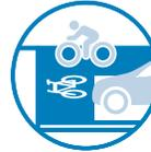
A designated area at the head of a traffic lane at a signalized intersection that provides bicyclists with a safe and visible way to get ahead of queuing traffic during the red signal phase.
