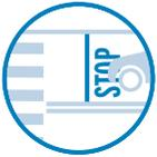
A stop bar placed ahead of the crosswalk at stop signs and signals reduces conflict with pedestrians from vehicles encroaching on the crosswalk.
