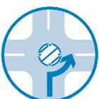
Installed at stop-controlled intersections to facilitate a circular flow at an intersection, which result in slower speeds through the intersection.
