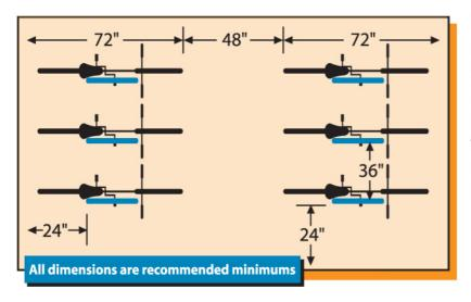
Six feet (72 inches) of depth should be allowed for each row of parked bicycles. Conventional upright bicycles are about 72 inches long and can easily be accommodated in that space. Some rack types will allow the racks to be mounted closer to a wall. This will not change the space required by the bicycle or the aisles.
