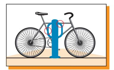
Like inverted "U" racks, bollard racks allow for two points of contact to properly park a bike.
