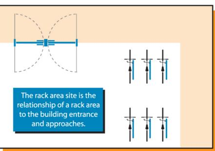
In the case of a bike rack, at some point the cyclist stops, dismounts, and walks the bike to the rack. The bicycle is attached to the rack and any cargo is removed. The cyclist now walks to the building carrying the cargo. Adequate space must be provided to allow for this transition.
