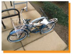
Normally, the handlebar and seat heights will allow two bicycles to line up side-by-side if one of them is reversed. If the rack elements are placed too close together, it becomes difficult to attach two bikes side-by-side.
