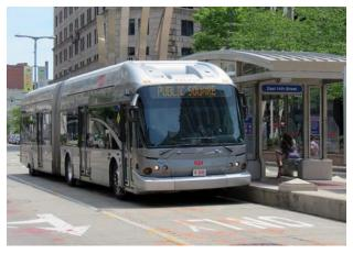
Bus Rapid Transit (BRT) is a specialized service that lets buses move through congested streets more quickly. It gives priority to buses at traffic signals, can include bus-only lanes, and makes it faster for passengers to get on and off buses.
