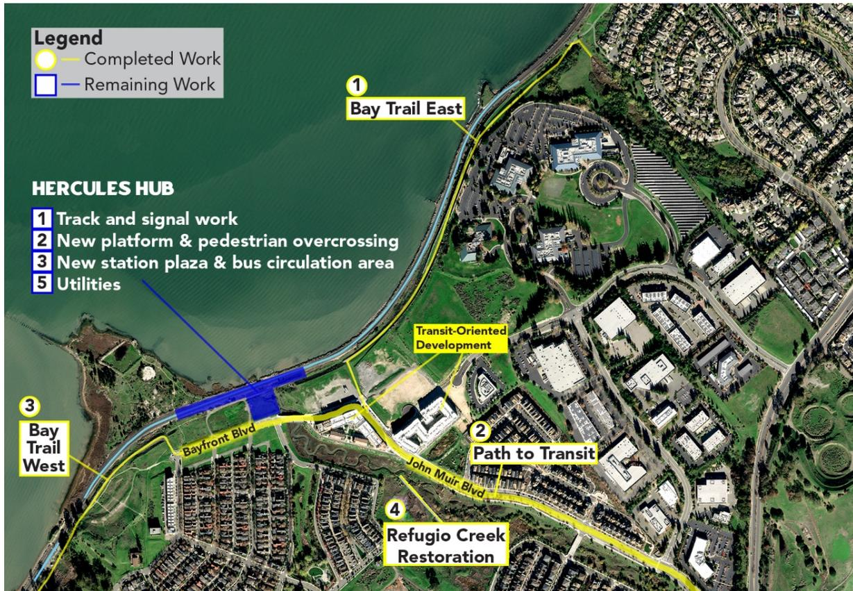
Figure 2: Completed and Remaining Project Components
