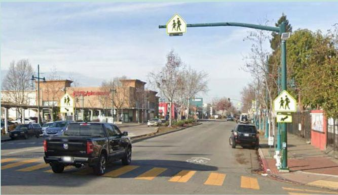
**Rectangular Rapid Flashing Beacons** are flashing lights that warn drivers when pedestrians are in the crosswalk.
